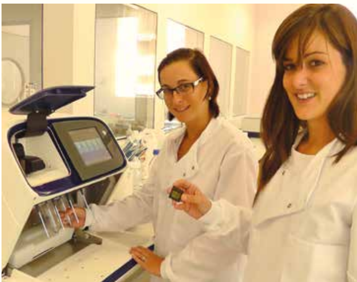
DNA encoding the exome is loaded onto a microchip and placed into the DNA sequencer . DNA can be sequenced within two days but data can take several weeks to analyse.
